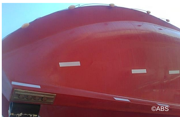
Lifeboat reflective tape replaced
