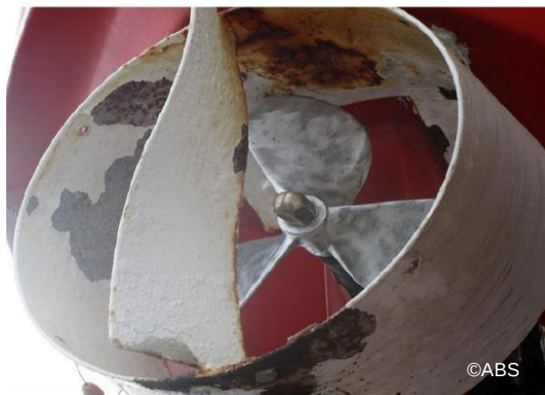
Lifeboat rudder corroded - before
