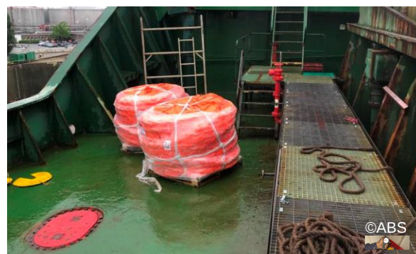
New mooring ropes provided
