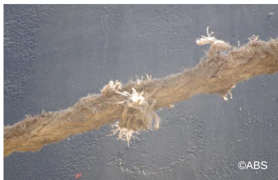
Mooring rope with broken strands
