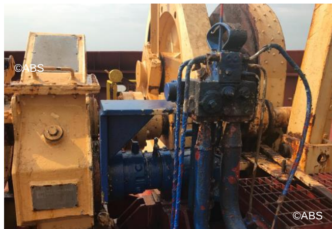
Damaged hydraulic motor for mooring winch replaced
