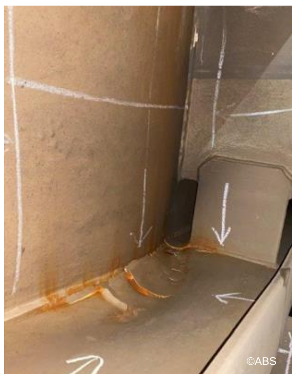
Internal structure buckled due to side shell contact damage
